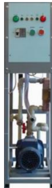
Cooling station CS-10 (dimensions: 300x900x600)
